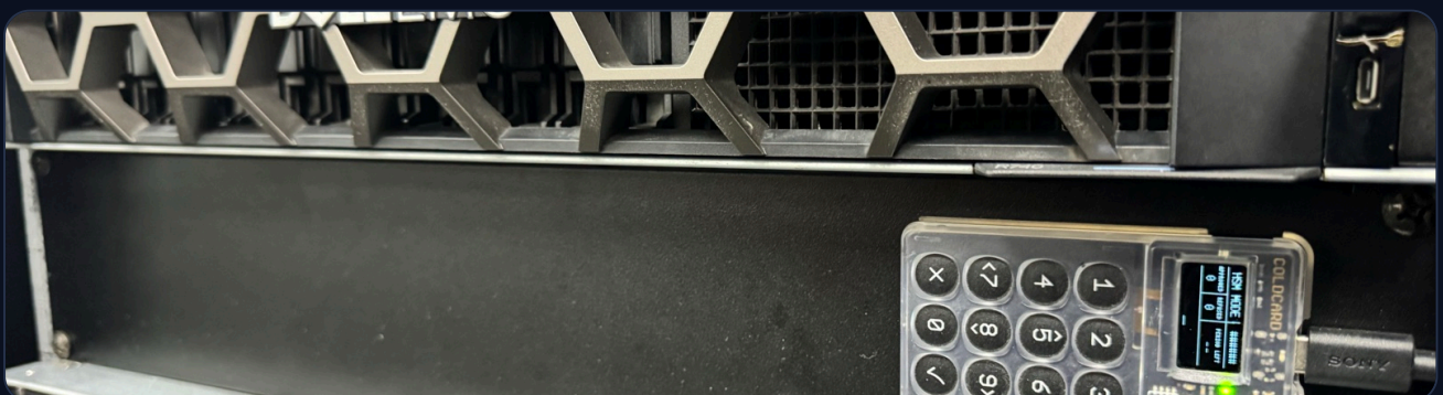
Real hardware. A Coldcard in HSM mode, signing on a host in the rack — one of three independent signers.
